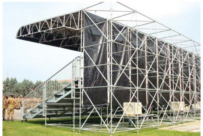
Possibility to create cantilevered roofing sizes from 4.70 m to 8.60 m using a specifically shaped lattice beam connected to a back wall made of MP Multidirectional scaffolding to protect grandstands and walkways.
